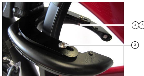
fig. 2: mounting spoke lock
